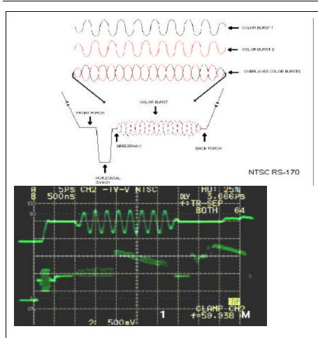
Figure 2: Color Burst and Composite Video Line (Single Shot, triggered on Both Fields, Line Number 64, zoom on burst)
