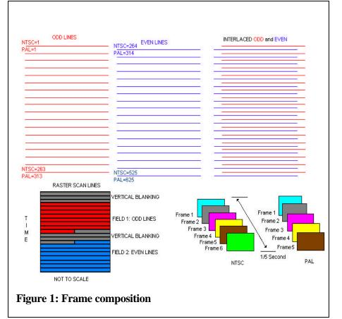
vertical blanking interval and others are for test, or special purposes. The electron beam(s) writing to the screen make two trips per frame. The first trip down the beam(s) "draw" all the odd-numbered lines of the frame, the second time down the even-numbered lines are drawn.
