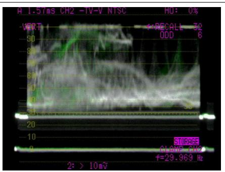
Figure 3: Composite Video; TV Line Trigger (Odd Field Line Number 6) displaying one full video Frame. Dynamic changes in white, persistence fade in green.
