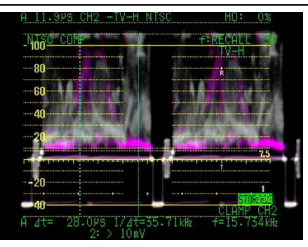
Figure 4: Composite Video 2H with EIA scales displayed on LA354 with Storage enabled (violet is stored trace, white is live feed).
